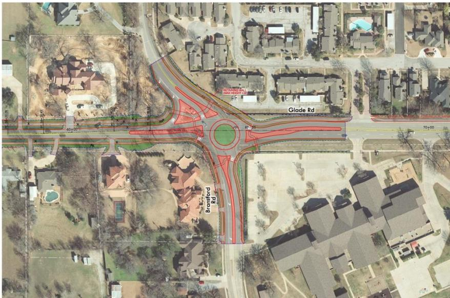
The Bransford roundabout would help address traffic flow issues at this intersection, particularly at peak hours. Construction on the roundabout is a priority for the summer of 2015, in order to minimize disruption during the school year.
