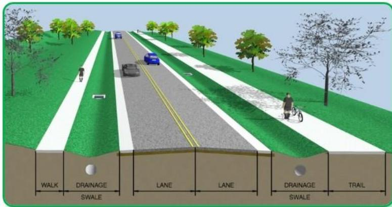
**Section 1 of Glade Road, River Bend Drive to Bransford Road, is proposed to remain a two-lane, asphalt roadway with left-turn lanes where warranted**
